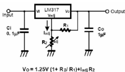
$C_i$  is required when regulator is located an appreciable distance from power supply filter.
