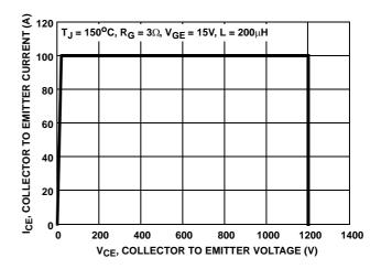
FIGURE 2. MINIMUM SWITCHING SAFE OPERATING AREA
