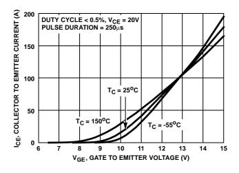
FIGURE 13. TRANSFER CHARACTERISTIC
