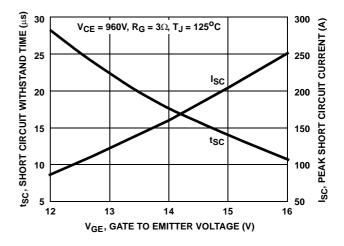
FIGURE 4. SHORT CIRCUIT WITHSTAND TIME
