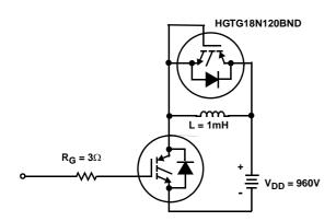
FIGURE 20. INDUCTIVE SWITCHING TEST CIRCUIT
