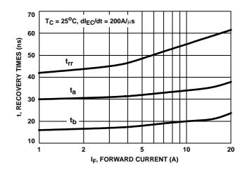
FIGURE 19. RECOVERY TIMES vs FORWARD CURRENT
