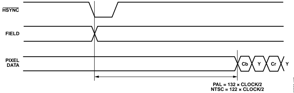
Figure 105. SD Timing Mode 1, Odd/Even Field Transitions (Master/Slave)
