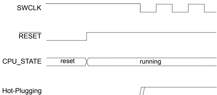
Figure 14-3. Hot-Plugging Detection Timing Diagram
