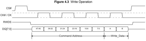
Host drives DQ[7:0] with Command-Address and Write Data
