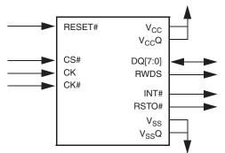
HyperFlash memories use the HyperBus low signal count, high-speed interface and combine the best features of Execute-In-Place (XIP) and Data Storage flash memories. This family has the fast random access of XIP flash along with the high density and fast program speed of Data Storage flash.
