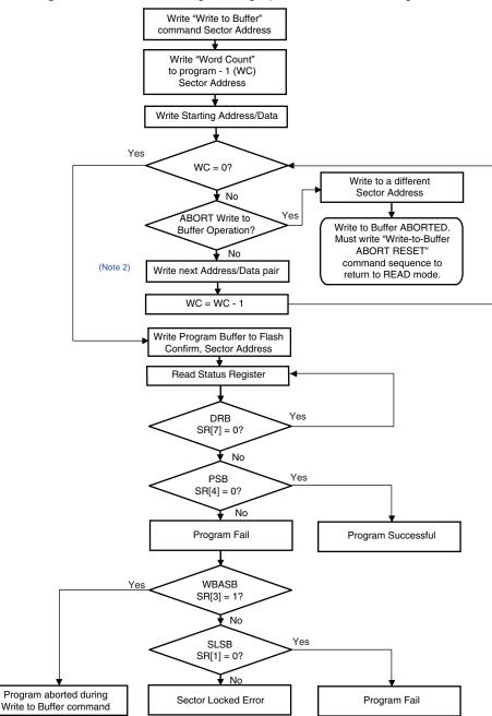
Figure 6.2 Write Buffer Programming Operation with Status Register
