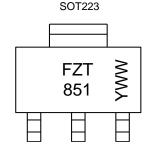
FZT 851 = Product Type Marking Code YWW = Date Code Marking Y or  $\overline{Y}$  = Last Digit of Year (ex: 5= 2015) WW or  $\overline{W}$ W = Week Code (01~53)
