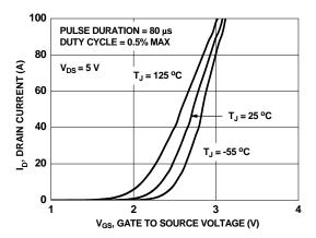
Figure 5. Transfer Characteristics
