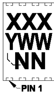
8-Lead TDFN (2x3) (MCP6N11)
