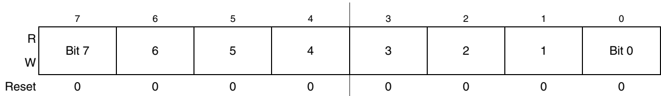
Figure 10-9. Timer x Counter Modulo Register Low (TPMxMODL)
