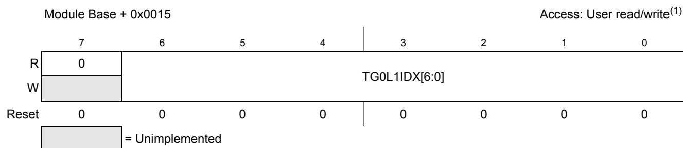
Figure 14-18. Trigger Generator 0 List 1 Index (TG0L1IDX)
