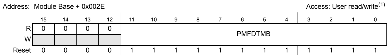
Figure 15-33. PMF Deadtime B Register (PMFDTMB)
