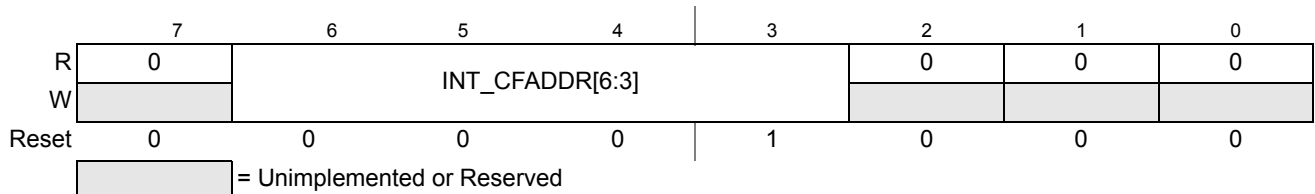
Figure 4-4. Interrupt Configuration Address Register (INT_CFADDR)
