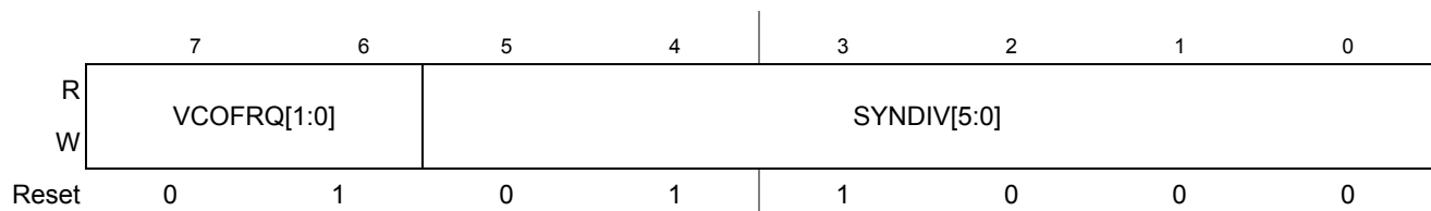
Figure 8-9. S12CPMU_UHV_V10_V6 Synthesizer Register (CPMUSYNR)
