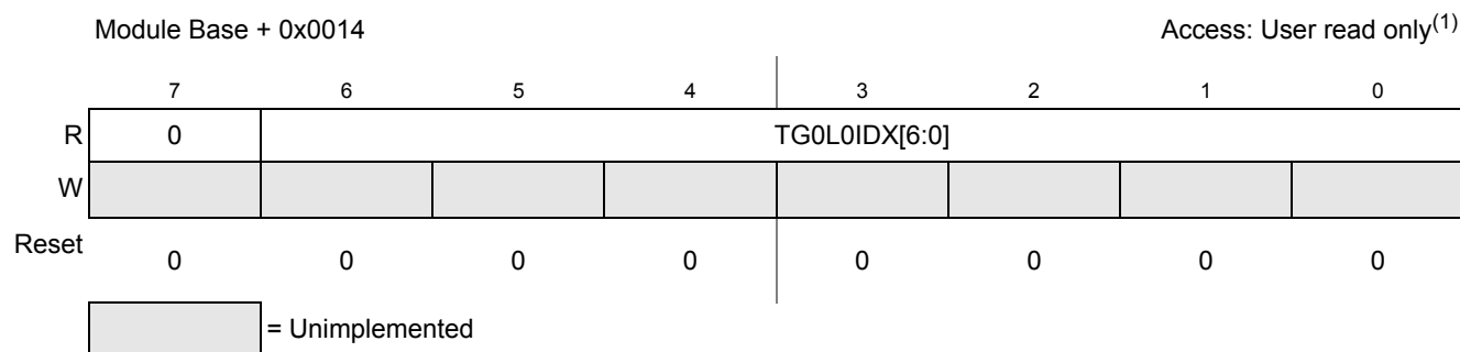
Figure 14-17. Trigger Generator 0 List 0 Index (TG0L0IDX)
