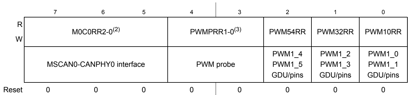
Figure 2-3. Module Routing Register 1 (MODRR1)
