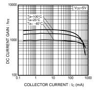
Fig.1 DC Current Gain vs. Collector Current
