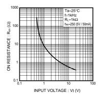
Fig.3 "ON" resistance vs. Input Voltage
