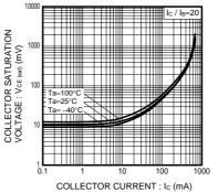
Fig.2 Collector-Emitter Saturation Voltage vs. Collector Current
