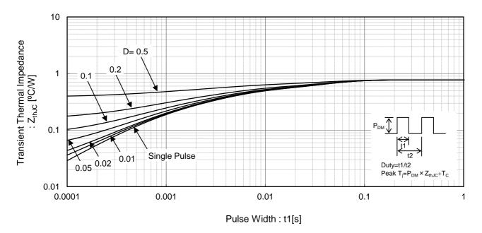
Fig.22 Diode Transient Thermal Impedance
