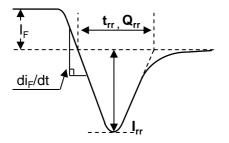
Fig.25 Diode Reverce Recovery Waveform
