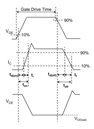
Fig.24 Inductive Load Waveform
