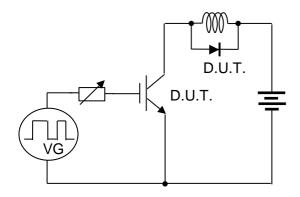
Fig.23 Inductive Load Circuit
