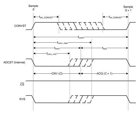
Figure 1. Conversion Cycle Timing
