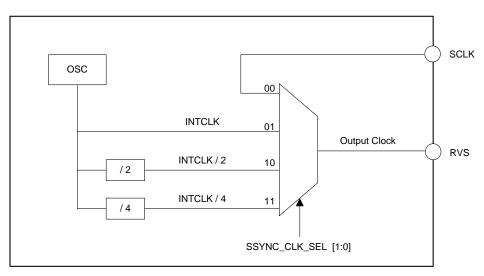
Figure 69. Output Clock Source Options With SRC Protocols
