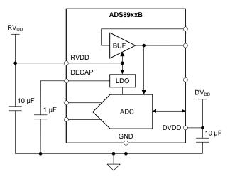
Figure 103. Power-Supply Decoupling
