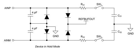
Figure 32. Input Sampling Stage Equivalent Circuit
