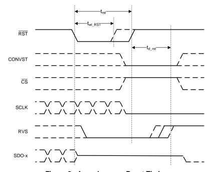
Figure 2. Asynchronous Reset Timing
