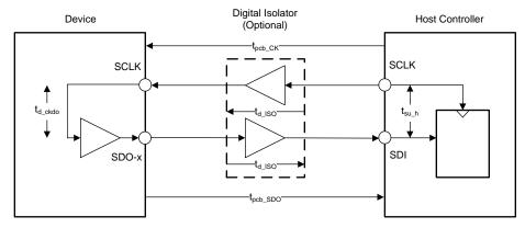
Figure 44. Delays in Serial Communication
