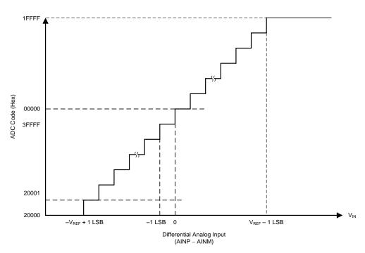
Figure 33. Differential Transfer Characteristics
