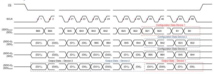
Figure 86. Three-Device, Daisy-Chain Timing
