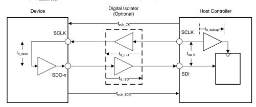
Figure 45. Delayed Capture
