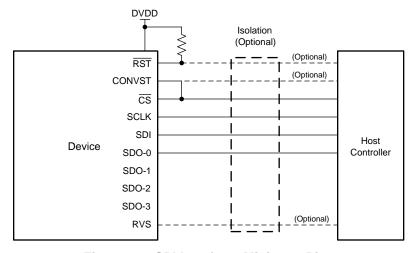
Figure 83. SPI Interface, Minimum Pins
