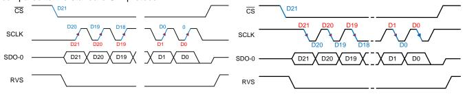
Figure 55. SPI-00-S-EDL Protocol, 22 SCLKs
