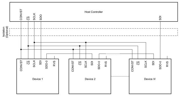
Figure 84. Daisy-Chain Connections
