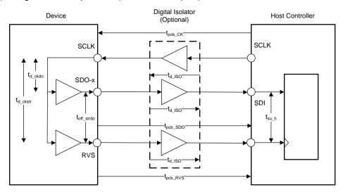
Figure 46. Delays in ADC-Clock-Master (Source-Synchronous) Mode
