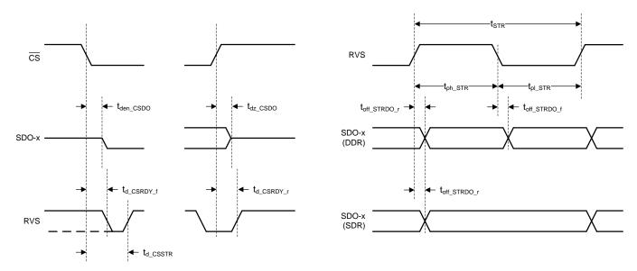
Figure 5. Source-Synchronous Serial Interface Timing (Internal Clock)
