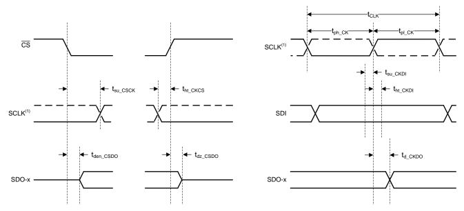
(1) The SCLK polarity, launch edge, and capture edge depend on the SPI protocol selected.
