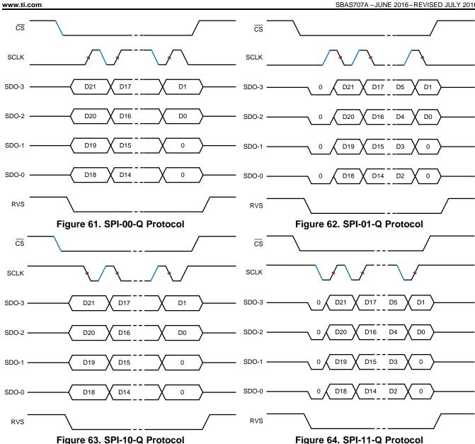
For SDI\_MODE[1:0] = 00b or 10b, the device supports an early data launch (EDL) option. Set SDO\_MODE[1:0] = 01b in the SDO\_CNTL register to enable the feature (see Table 8). Setting SDO\_MODE[1:0] = 01b has no effect if  $SDI_MODE[1:0] = 01b$  or 11b.
