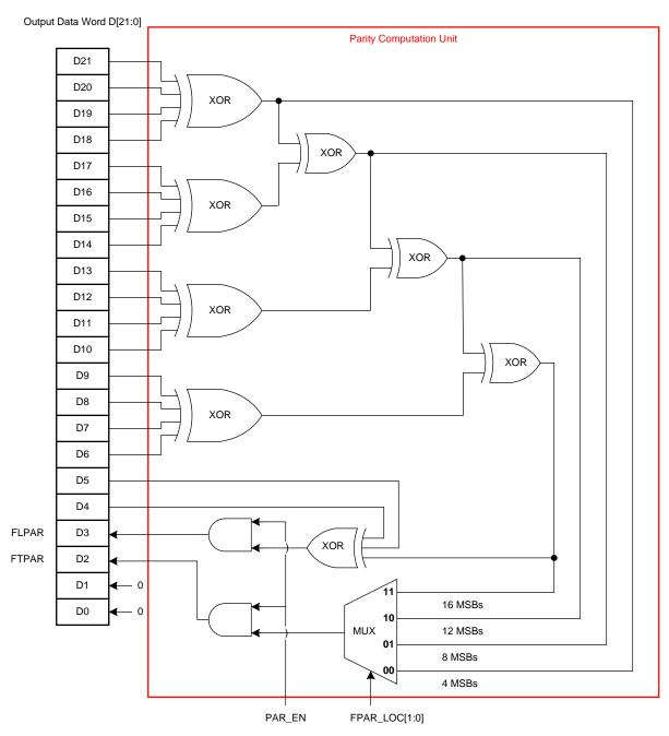
Figure 39. Parity Bits Computation
