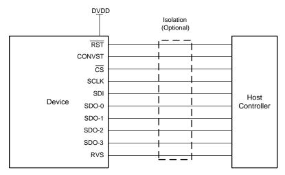
Figure 82. MultiSPI Digital Interface, All Pins
