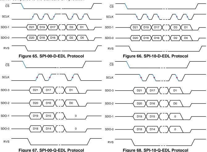
When using any of the SPI-compatible protocols, the RVS output remains low throughout the data transfer frame; see the *Timing Requirements* and Switching Characteristics tables for associated timing parameters.
