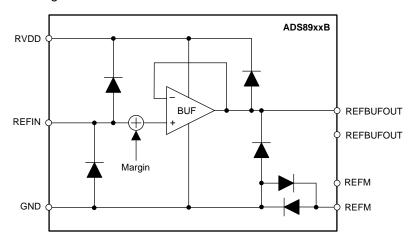
Figure 29. Internal Reference Buffer Block Diagram
