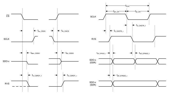
Figure 4. Source-Synchronous Serial Interface Timing (External Clock)
