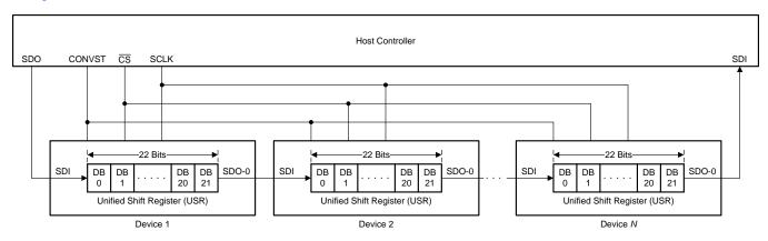
Figure 85. Unified Shift Register
