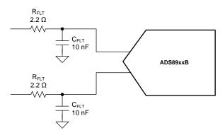
Figure 99. Charge Kickback Filter Configuration
