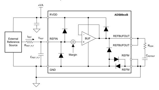
Figure 30. External Connections for the Internal Reference Buffer
