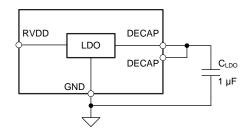
Figure 28. Internal LDO Connections
