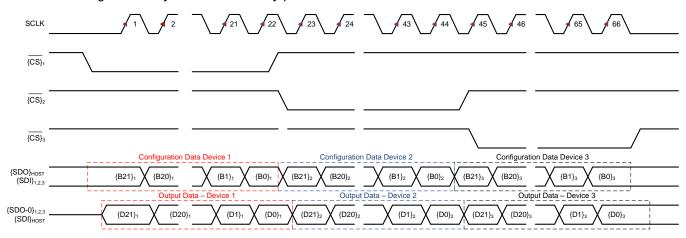
Figure 88. Three-Device, Star Connection Timing
