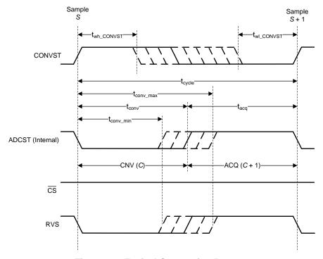
Figure 37. Typical Conversion Process
