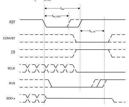
Figure 36. Asynchronous Reset
