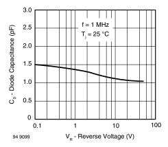
Figure 4. Diode Capacitance vs. Reverse Voltage
