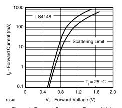
Figure 1. Forward Current vs. Forward Voltage
