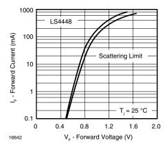
Figure 2. Forward Current vs. Forward Voltage
