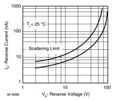
Figure 3. Reverse Current vs. Reverse Voltage
